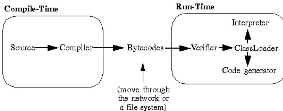
The verifier acts as a gatekeeper by preventing the execution of imported code until it has passed the verifier's tests. When code verification is complete a number of important properties of the code are known:
