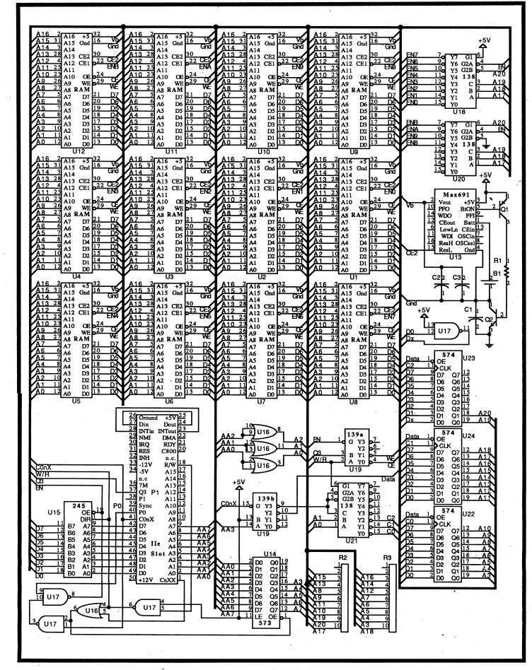
(R2, R3) pull address lines A3 thru A20 high. This means that when you read or write to a latch, you are also reading or writing to the eight (8) highest locations in SRAM.
